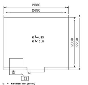
Supply voltage: 220 V/1N ph/50 Hz Electrical power, max: 1.96 kW
